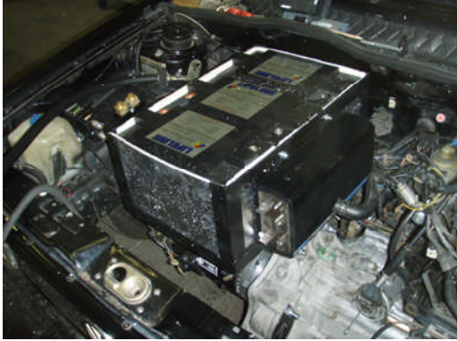
Before: motor and batteries installed
